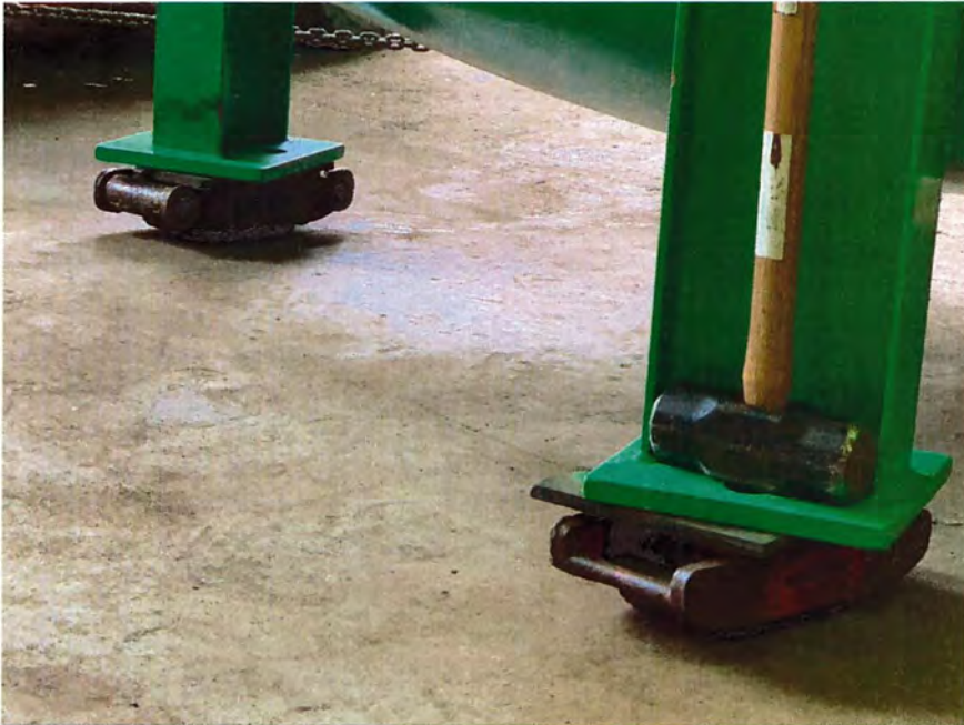
Heavy-Duty Rollers on each foot support nearly 3-Tons x 4
